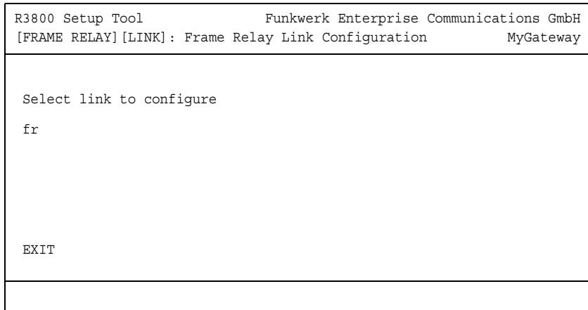
The **FR → LINK CONFIGURATION** menu contains the settings relating to layer 2 of the Frame Relay interface.
