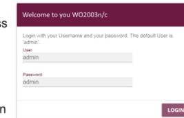
All devices are shipped with the same user names and passwords. As a result, they are not protected against unauthorised access. Make sure you change the password to prevent unauthorised access to your device. Go to **System Management** → **Global Settings** → **Passwords**. Enter a new password for **System Administrator Password**. Click **OK**. Save the configuration by clicking on the **Save Configuration** button in the header.
