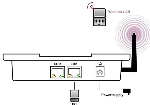
When setting up and connecting, carry out the steps in the following sequence:
