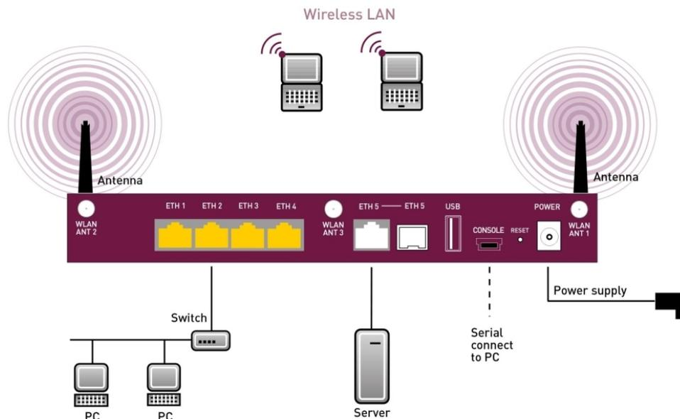
Fig. 6: Connection options using the example of **bintec RS120wu**
