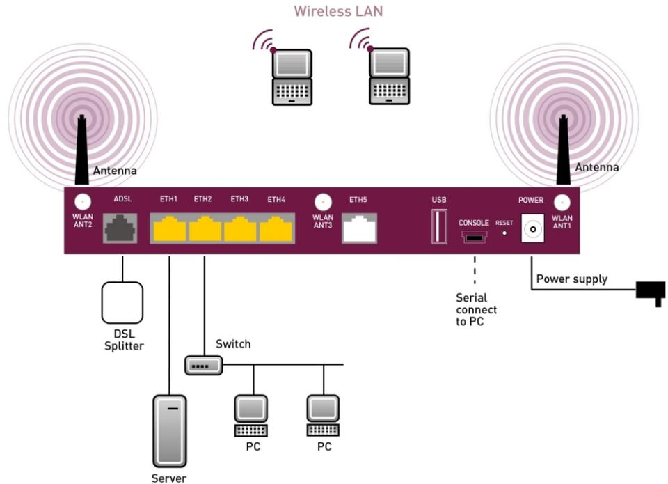
Fig. 11: Connection options using the example of **bintec RS230aw**
