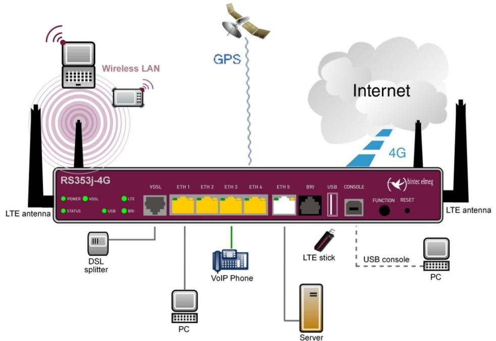
Fig. 2: Connection options using the example of **bintec RS353j-4G**
