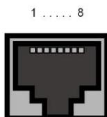
Fig. 24: ISDN S0 BRI interface (RJ45 socket)
