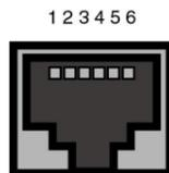
Fig. 23: ADSL interface (RJ11)
