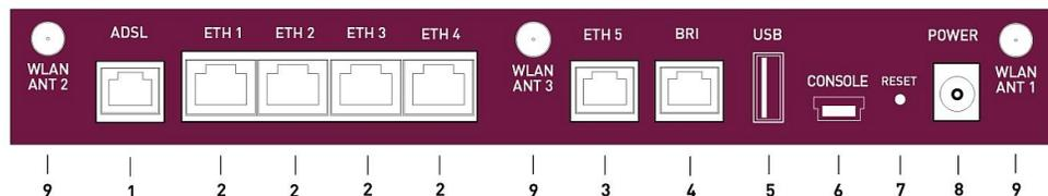
Fig. 17: **bintec RS232jw** rear panel
