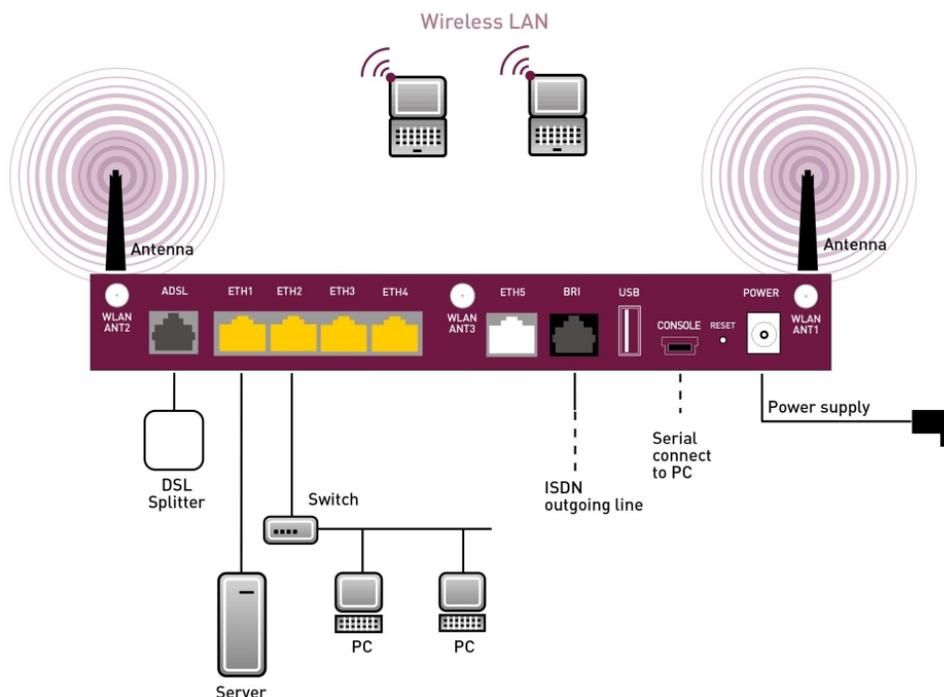
Fig. 16: Connection options using the example of **bintec RS232jw**
