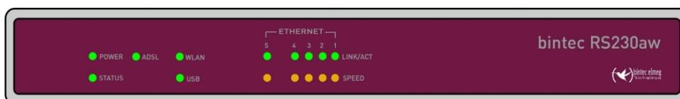
Fig. 15: Arrangement of LEDs
