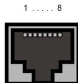
Fig. 22: 10/100/1000 Base-T Ethernet interface (RJ45 connector)
