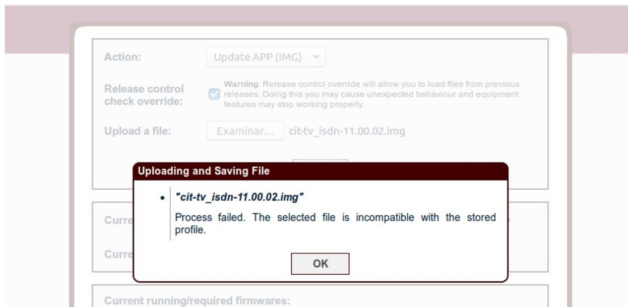
Here, we were trying to upload an "isdn" profile file in a device that does not support it.
