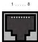
Fig. 23: Ethernet 10/100 Base-T interface (RJ45 socket)
