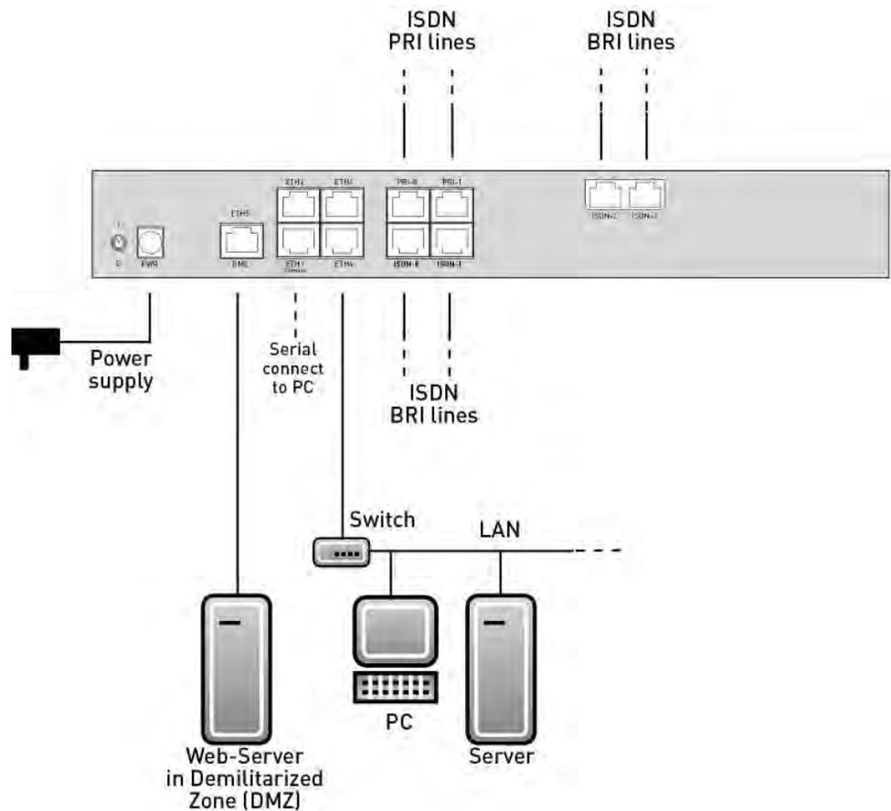
Fig. 4: Connection options using the example of **R41000**
