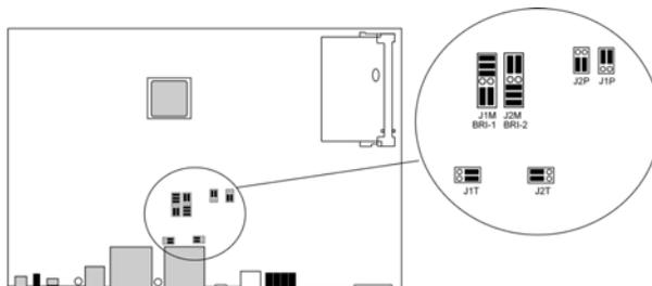
Insert the link plugs for interfaces BRI-1 and BRI-2 as shown in the following figure:
