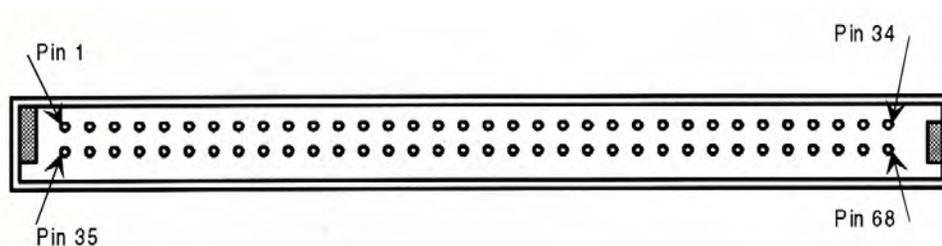
Fig. 26: 68-pin CardBus slot for UMTS modem card
