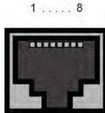
Fig. 28: SHDSL interface (RJ45 connector) **bintec R3400**
