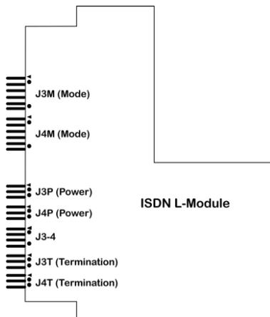
Insert the link plugs for interfaces BRI-3 and BRI-4 as shown in the following figure:
