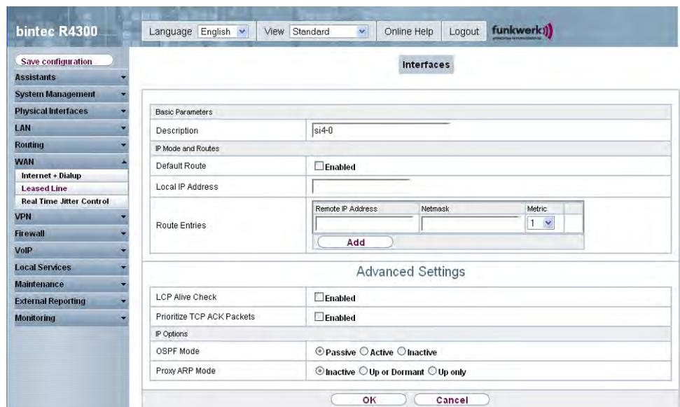
The screenshot shows the configuration page for a WAN Leased Line interface on a bintec R4300 device. The interface is titled "Interfaces" and is divided into "Basic Parameters" and "Advanced Settings".
