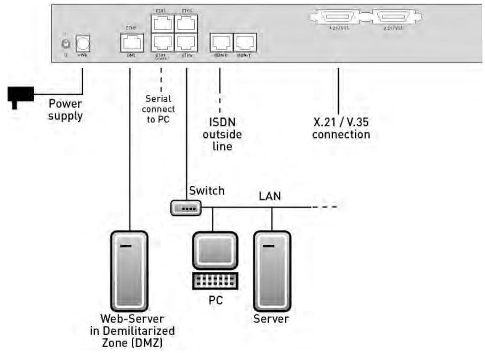
Fig. 3: Connection options using the example of R43000
