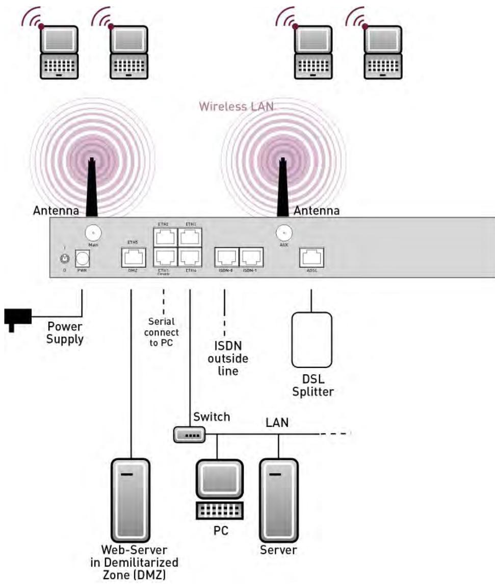
Fig. 2: Connection options using the example of R3000w
