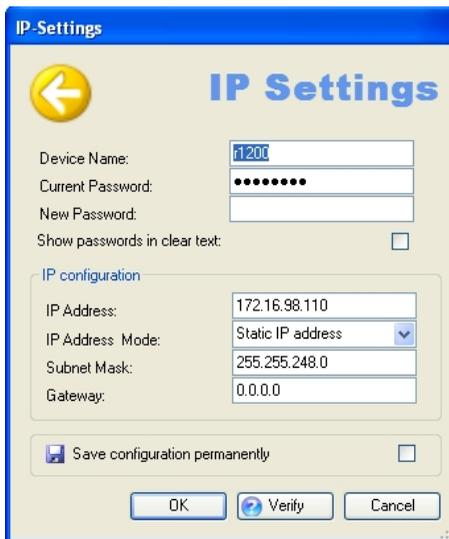
Fig. 25: IP address assignment with the **Dime Manager**
