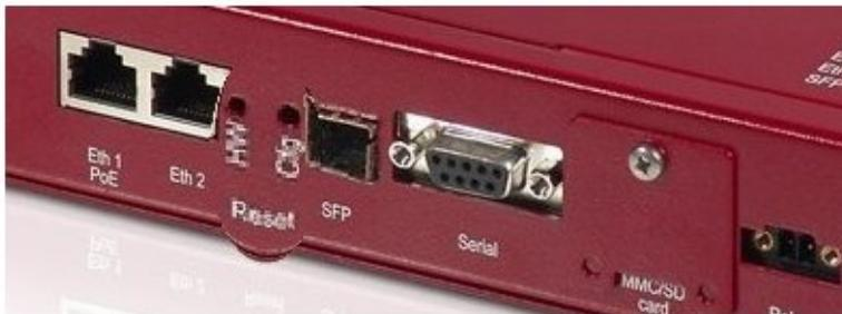
Fig. 17: Underside of the **bintec Wlx040n** with the HW and Cfg reset buttons
